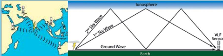
*A network of sensors operating in the Very Low Frequency (VLF) band and measuring horizontal magnetic fields of radio impulses generated by return strokes and large cloud pulses produce GLD360 data.*
